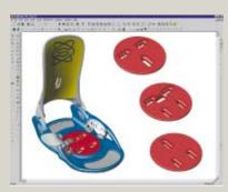
Using SolidWorks, configurations of products, assemblies, and product families can be created and managed from the original design, such as the multiple bolt patterns shown here for a snowboard binding.
